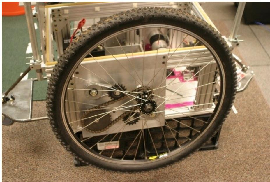
**Figure 1 – Revised drivetrain and suspension**
